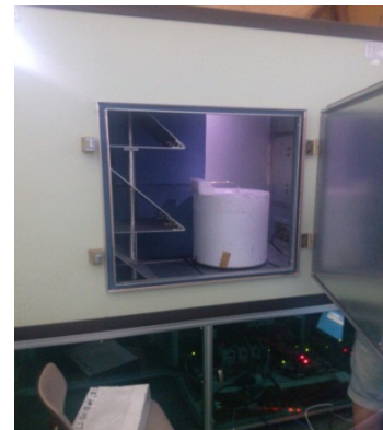
Fig. 1. A validation model for the power balance method using the reverberation chamber located at Korea Advanced Institute of Science and Technology.
