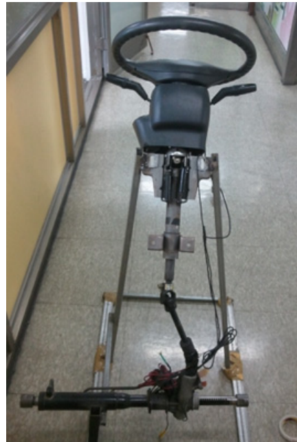
[Fig. 9] Jig for Performance Evaluation
