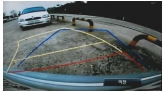
[Fig. 2] Example of Reverse Parking Guidance System UI
