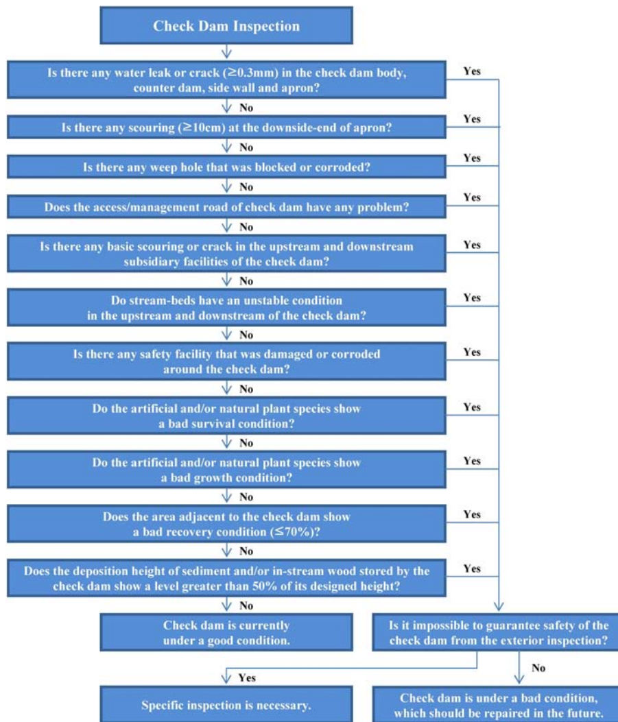
Fig. 2. Flow chart of the check dam safety inspection.
