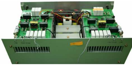
Fig. 12. Picture of 20kW converter block consisted of two 10kW modules
