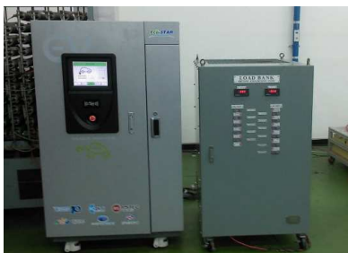
(b) Test setup for battery charging simulator
