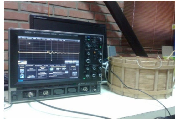
Fig. 2. The tested distribution 20kV transformer winding
