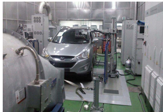
Fig. 2 Chassis dynamometer for vehicle emission test
