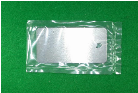
Fig. 4. Anti corrosion test specimen
