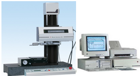
[Fig. 4] Stylus type surface roughness tester
