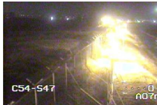
[Fig. 2] The CCTV screen by counterlight
