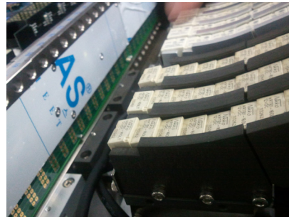
[Fig. 2] Relay are not horizontally stand
