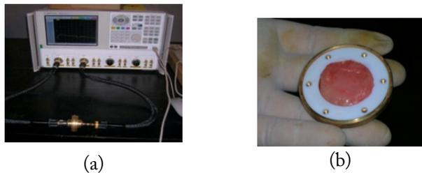
Fig. 3. Two-port measurement to determine the electrical properties of human breast and tumor tissues: (a) measurement setup and (b) tissue in the probe.
