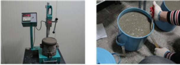
(a) Setting time test (b) Bleeding test
