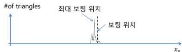
(e) Distribution of triangles built by DT for the location of vanishing point x_v .
