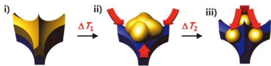
Fig. 11. Proposed mechanism for the formation of gold nan-triplet on AAO by dewetting. 14)
