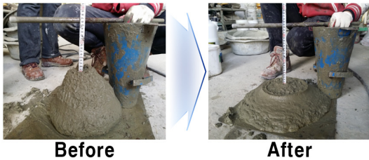
Fig. 3. Improving material property using form concrete Improvement of material property using form concrete
