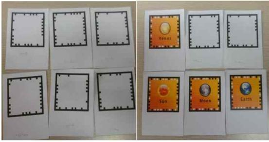
(Figure 10) Frame Marker (a) Marker with the edges of the sawtooth shape (b) Designed frame marker
