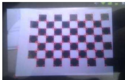
(Figure 6) Corner points detected from the image using mobile devices checkerboard
