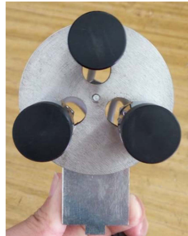
Fig. 6. (Color online) The arrayed EC sensors.
