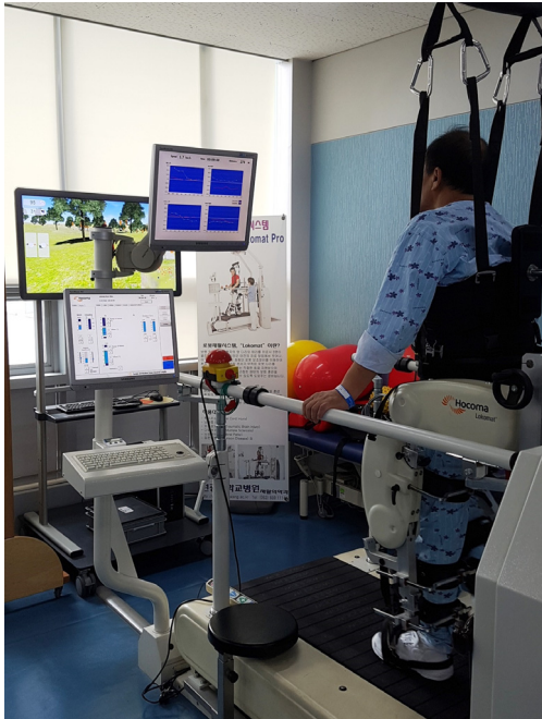
Fig. 2. Virtual reality based robot assisted rehabilitation using Lokomat.
