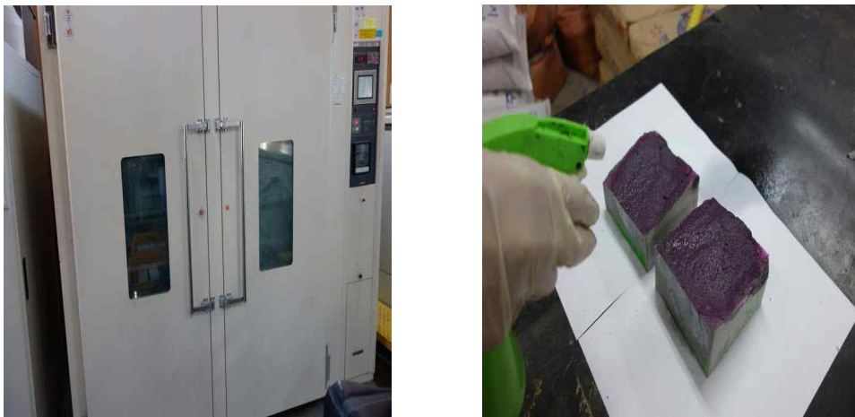
Fig. 3. Photos of carbonation resistance test of concrete with modified sulfur.
