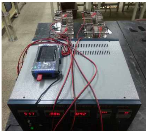
Fig.1. Photos of rapid chloride penetration test to determine chloride penetrability of concrete by KS F 2711.
