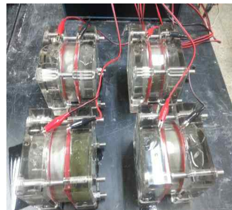
Fig.1. Photos of rapid chloride penetration test to determine chloride penetrability of concrete by KS F 2711.
