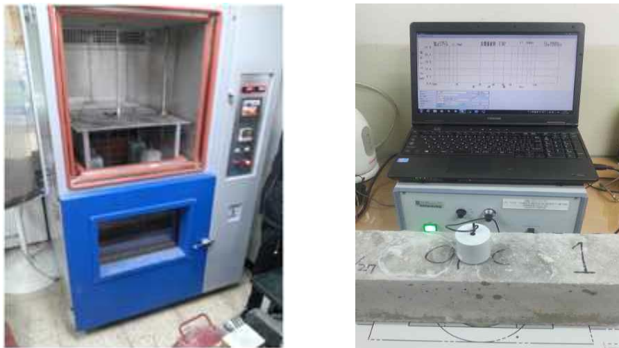
Fig. 4. Photos of rapid freezing and thawing test. (a) Test chamber, (b) Measuring dynamic elastic modulus of specimen
