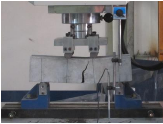
Fig. 11 Test for modulus of rupture
