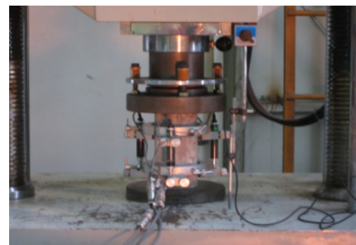
Fig. 5 Instrumentation for measurement of elastic modulus
