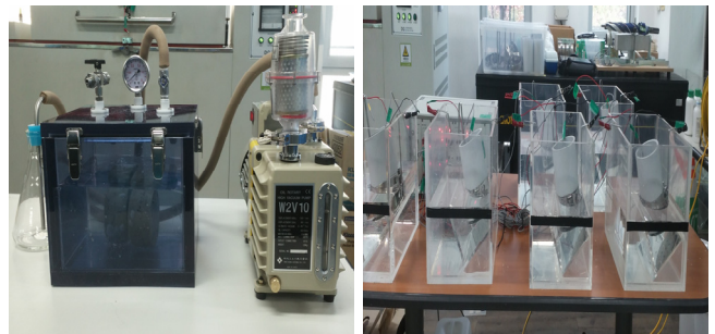
Fig. 4 Non-steady-state migration experiment
