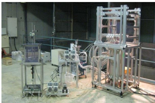
Fig. 8. Recycle system of the polishing agent by using HGMS and Magneto-Archimedes method.
