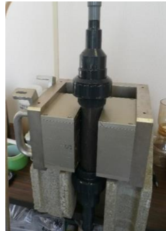
Fig. 9. The experiment of soil decontamination by HGMS in Fukushima.
