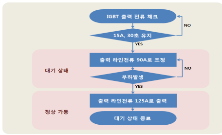
Fig. 7. algorithm of current output control
