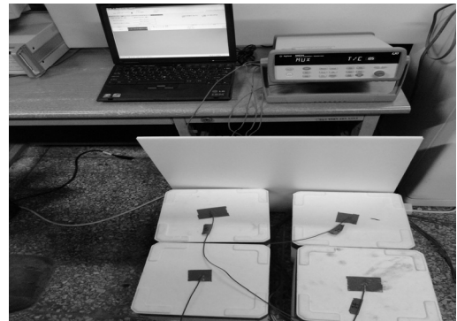
Fig. 4 Apparatus of simplified adiabatic temperature rise test
