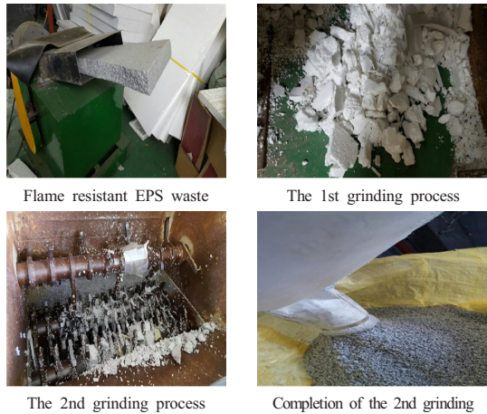
Fig. 2. Flame resistant EPS waste grinding process
