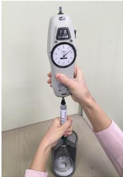
Fig. 9. Apparatus for the measurement of activation forces of autoinjector
