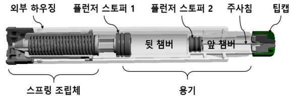
Fig. 2. Detailed structure of ATNAA(cited from ref. 3)
