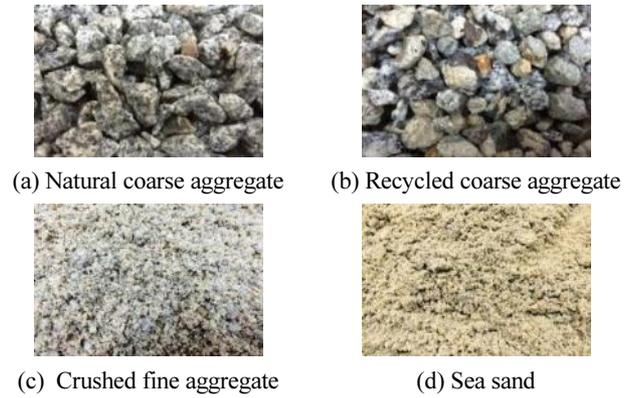
Fig. 1 Aggregates used in concrete mixtures
