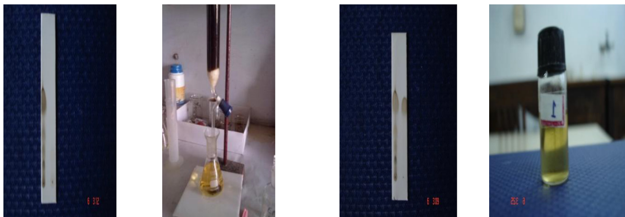
Figure 1 Isolation of acyclic isoprenoid from the butanolic fraction of Semecarpus anacardium seeds by using TLC and column chromatography. (Mobile Phase: hexane : ethyl acetate in the ratio of 8 : 2).
