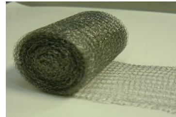
Fig. 2. The ferromagnetic thin wire mesh filter. The wire diameter is 0.1 mm SUS430.
