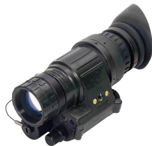
Fig. 3. Image Intensifying(Night Vision) Device[4]
