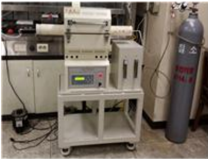
Fig. 3. Test Rig for testing of Annealing conditions.
