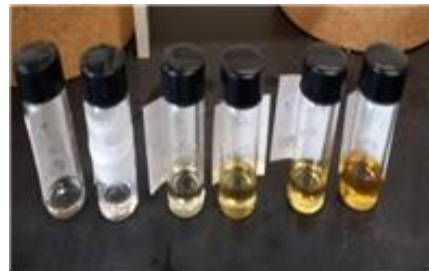
Fig. 6. Thermal denaturation of Rolling Oil depend on temperature.
