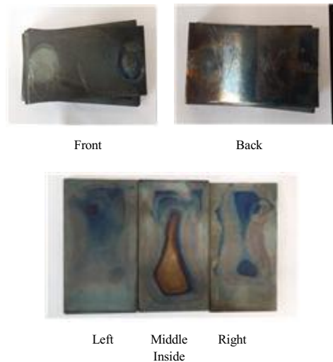
Fig. 9. Surface condition of specimen after annealing at 700 ℃.
