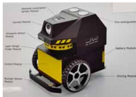
Fig. 6. Implemented autonomous running fire monitoring robot.
