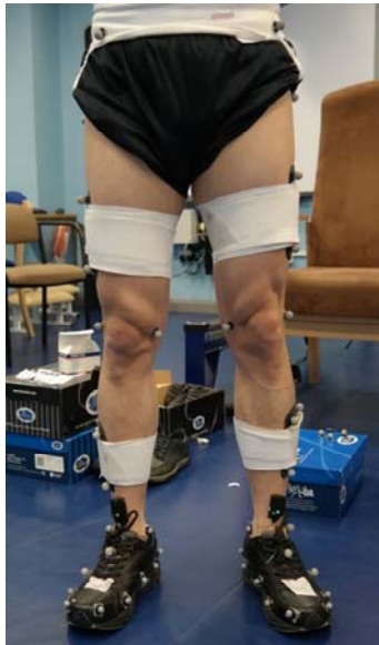
Fig. 1. Reflective marker sets on lower extremities for static calibration and dynamic motion capture
