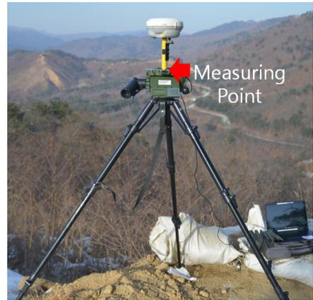
Fig. 8. Positioning by VRS RTK
