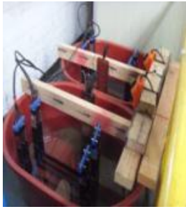
Fig. 6. Experimental set up of water absorption test
