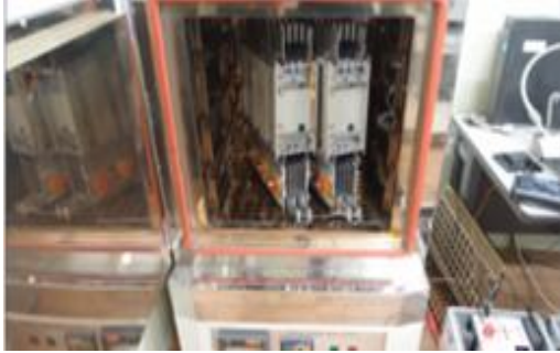
Fig. 3. Experimental set up of thermal accelerating aging test
