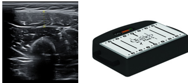
Fig. 1. Image of ultrasound (E-Cube15Ex) for test of muscle thickness (Lt) and Galileo® Med S (Rt).
