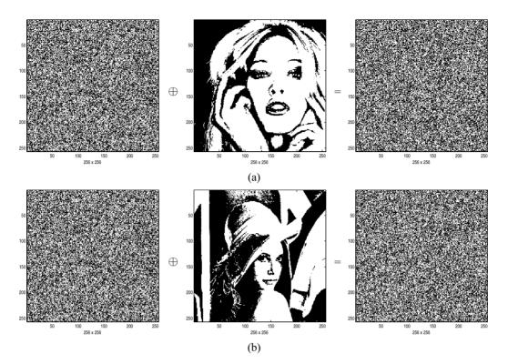
FIG. 6. Pre-encrypted private-key data images before the phase-shifting digital holographic encryption: (a) user A's pre-encrypted data  $p_A \oplus g$  by XOR operation of  $p_A$  and g, and (b) user B's pre-encrypted data  $p_B \oplus g$  by XOR operation of  $p_B$  and g.
