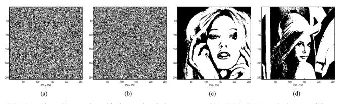
FIG. 5. Binary data and images to be used for the secret-key-sharing cryptosystem ( $256 \times 256$  pixels): (a) a randomly generated binary data image as the generator *g*, (b) a randomly binary data image as the encryption common key *k*, (c) a binary image as user A's private key *p<sub>A</sub>*, and (d) a binary image as user B's private key *p<sub>B</sub>*.
