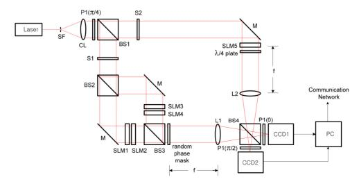
FIG. 3. Optical schematic for the proposed secret-key-sharing cryptosystem using two-step quadrature phase-shifting digital holography.
