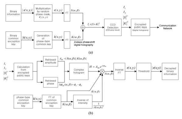
FIG. 4. Flow charts for the two-step phase-shifting digital holographic cryptosystem: (a) encryption, (b) decryption.
