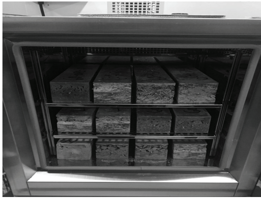
(a) Specimens fixed in constant temperature and humidity chamber
