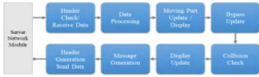
Fig. 5. Data flow sequence in an object
