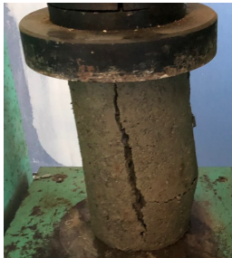
Fig. 3. Compressive strength test sight
