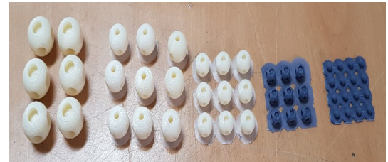
Fig. 2. Coarse aggregates made with 3D printer
