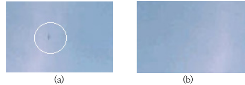
Fig. 11. Visual Stealth Experiment for a UAV using Electro-luminescent System[21] (a) System-off (b) System-on
