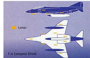
Fig. 9. Installation of Light Lamps for F-4[14]
