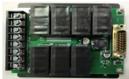
Fig. 10. The circuit board for air conditioner with relays
