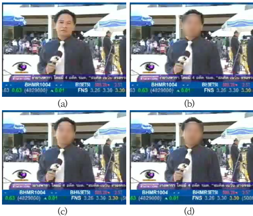
Fig. 3. Privacy area blocking (a) Original image (b) Blocking(t+1) (c) Blocking(t+2) (d) Blocking(t+3)
