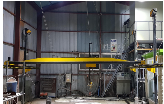
Fig. 1. Concrete 3D printing machine
