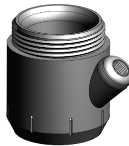
Fig. 2. Concrete 3D printing nozzle
