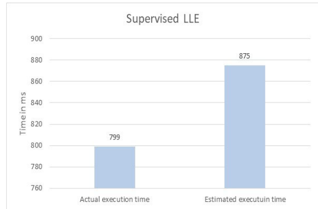
Fig. 29 Comparison between the actual and the estimated execution time for supervised LLE
