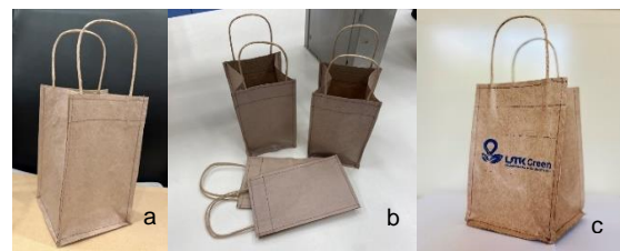
Figure 9: Packaging prototype from water hyacinth for the survey (Source: compiled by authors)
