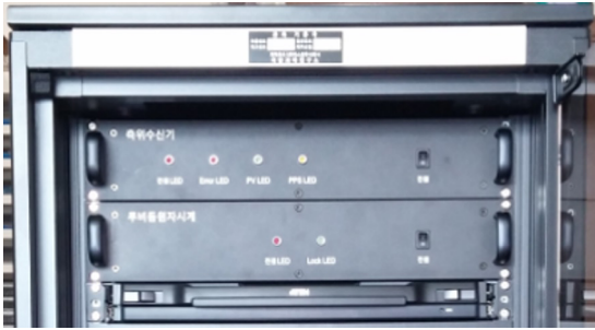
Fig. 6. User equipment with PPS and SPS GPS receivers.
