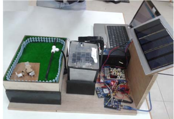
Fig. 5. The laboratory-developed prototype of fully automated irrigation system.
