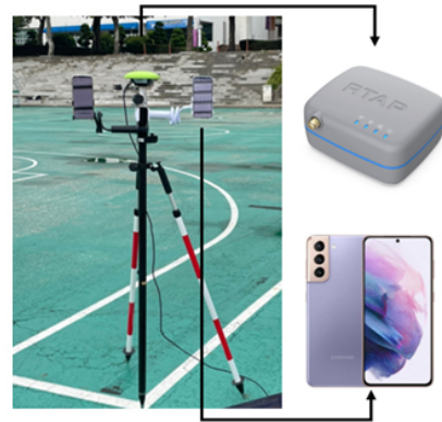
Fig. 1. The setup of RTAP2U and Galaxy S21+ during data collection.
