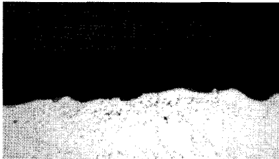
(b) Interfacial failure in opening-mode loading.
